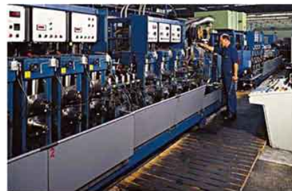
This is the type of installation, where Ampco 25 forming rolls are used for the production of stainless steel tubes (above: welding station).
