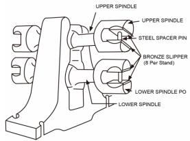
METHOD OF MANUFACTURE: Sand cast and finish machined or cast-to-size to 1/32" tolerance
