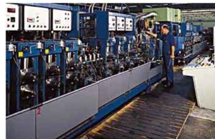
This is the type of installation, where Ampco 25 forming rolls are used for the production of stainless steel tubes (above: welding station).
