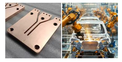
AMPCOLOY<sup>®</sup> 972 is used in a wide variety of industries. In the automotive sector, this versatile alloy excels in resistance welding tips and electrode caps, where its exceptional wear resistance and electrical conductivity are invaluable. This high copper alloy consistently delivers reliable results, demonstrating its adaptability to a wide range of applications.
