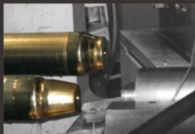
Expansion of tube in 2 steps, with mandrel in AMPCO® 25.
