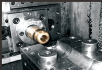
End forming on stainless steel tube with AMPCO® 25 mandrel.
