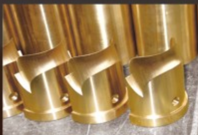
Insert wiper dies in AMPCO® 18.
