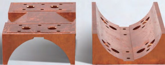
Contact Plates: Used in iron alloy furnaces, they are provided with cooling channels. Made of copper-Zinc (85% - 15%) or in high conductivity pure copper
