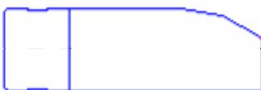
**Formed plug mandrel** - Used for heavy walled tube and pipe on tight radius.
